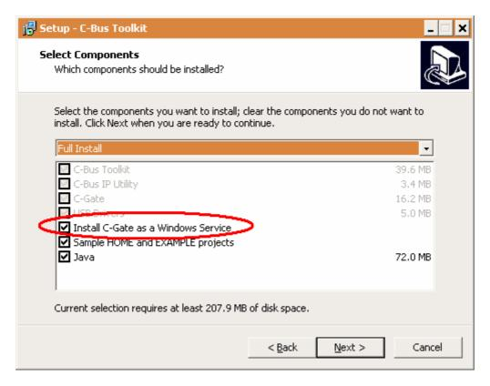
The C-Gate service will automatically start after installation and each time the computer is rebooted.
